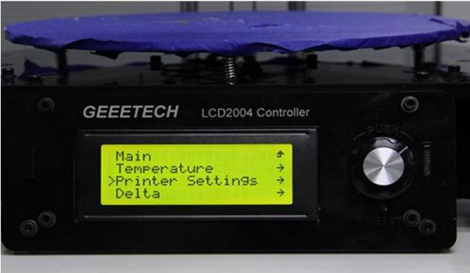
Scroll down to Motor Dir. If X axis direction is reversed, you can choose the X motor Dir, press the knob,
