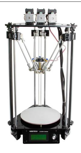
**Note:** the origin point is the corner of the platform when printing. So when the printer is at home position, the coordinates of X/Y axis are: X=0mm, Y=0mm, Z=220mm. As a result:
