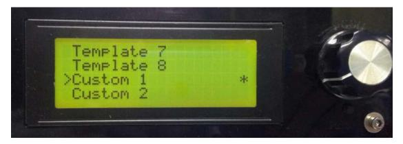
Note: the "\*" after the template means the current template you are choosing and using. System will follow your last chosen operation by default.
